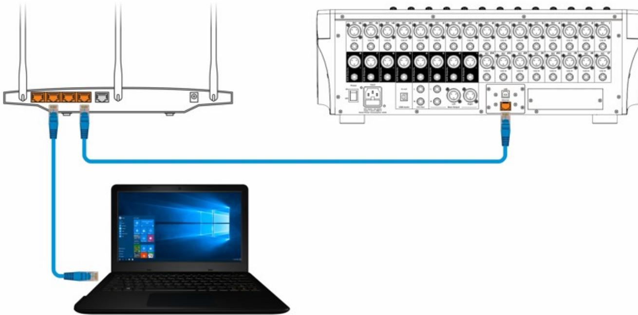
2 - Wireless mixer and computer: Connect the EtherNet port of the DM24.8 device to a "Router" port. Find the name of the network that corresponds to the "Router" you are using on the computer's wireless system and connect via Wi-Fi. That way the computer will see the DM24.8 mixer.
