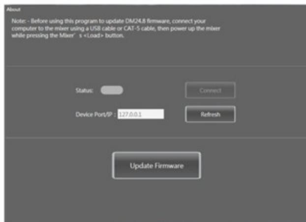
2.2 Click Refresh button to scan the device. And then the IP or COM address of the device will appear, depending on the connection method being used. Click the Connect button. If the status light is green, the device is connected correctly.
